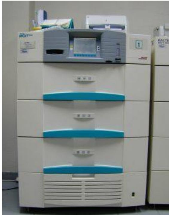
**Figure 5:** Automate Bactec MGIT 960.
